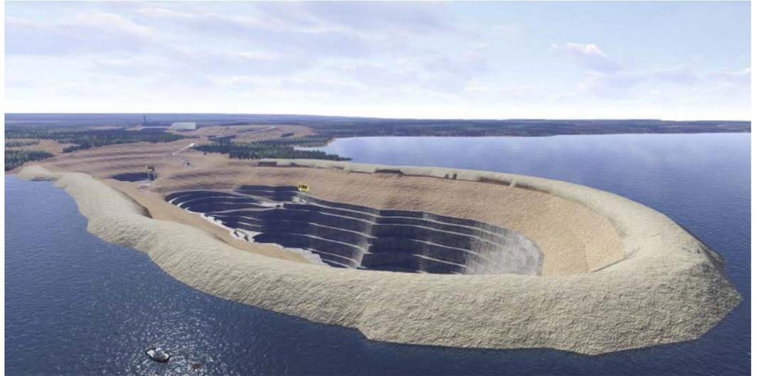
*Schematic view of the proposed pit and dyke*
