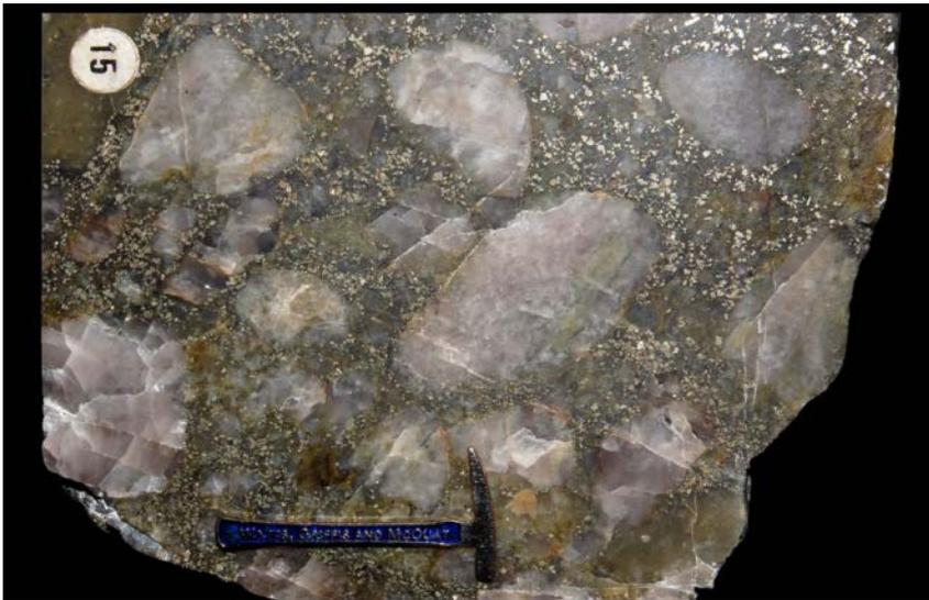
Uranium-containing quartz-pebble conglomerate with pyrite
